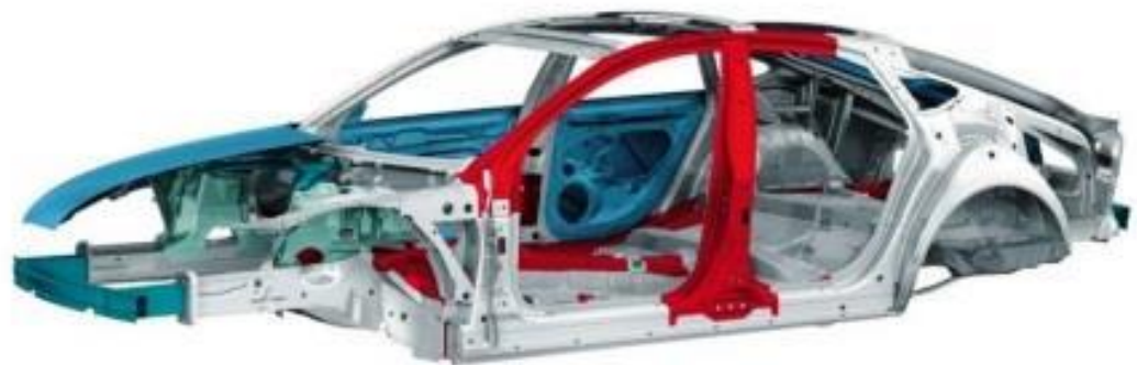
Hybrid Steel-aluminium body structure of the Audi A7 Sportback (Source: Audi)
